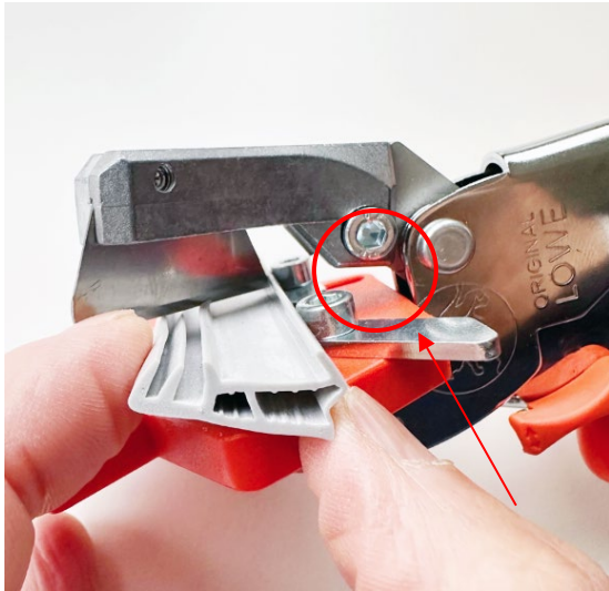
Tilting the seal during notching
