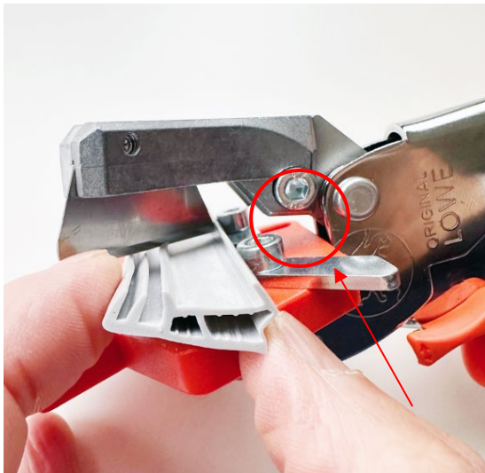
Tilting the seal during notching
